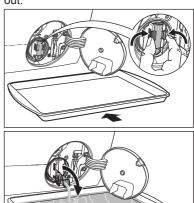
When the container is full of water, put the drainage duct back again and empty the container. Do step 3 again and again until no more water flows out from the drain pump.
