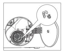
Make sure that the impeller of the pump can turn. If this does not occur, contact the service centre.
