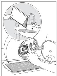
4. Push back the drainage duct and turn the filter counter-clockwise to remove it.
