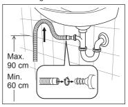
Push the drain hose onto the spigot and secure with a clip, ensure a loop is formed in the drain hose to prevent waste from the sink entering the appliance.  Directly into a drain pipe, at a height of not less than 60 cm and not more than 90 cm.
